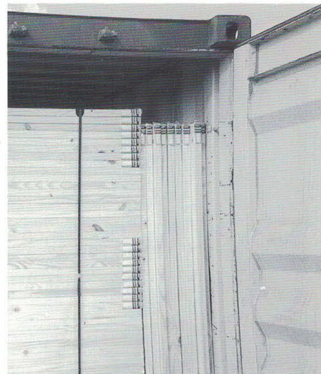
Timber doors packed in the potential heat trap of an enclosed steel container.
