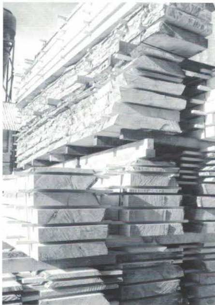
Selected British grown pine drying for the production of gates
