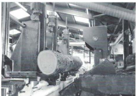
One of the larch logs from previous picture set on the head-rig ready for conversion
