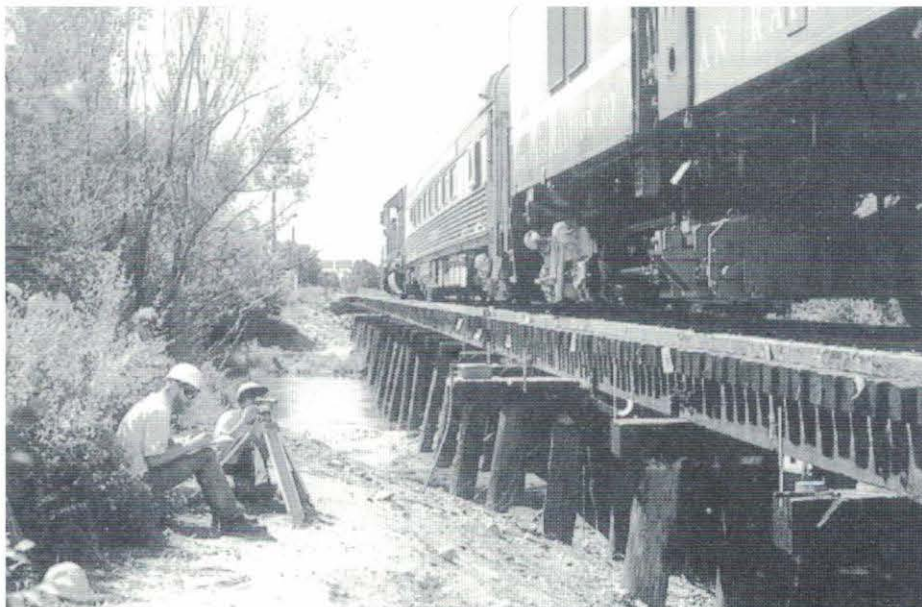
Field testing 31-span bridge for deflection, strain, accelerations, etc.
