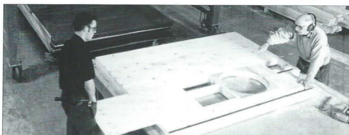
The manufacture of timber frame panels using structural softwood plywood
