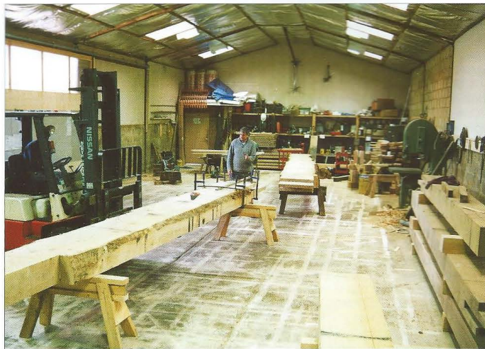
General view of one of the Green Oak Company Workshops and the fork lift truck (FLT) being used to assist in the centering a bridge beam over the datum line.
