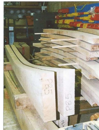
Curved members stored ready for assembly. Locations for such members can be seen on the plan.
