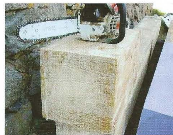
300 x 300 section of Pine cut after microwave drying revealing no drying checks (temperature was -15° C thus the 'white' look to the end grain!)
