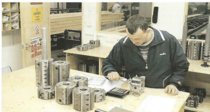
Checking tooling tolerances in new tool room, Lingfield depot
