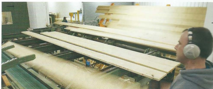
Quality selection on the new high speed production line, Lingfield depot
