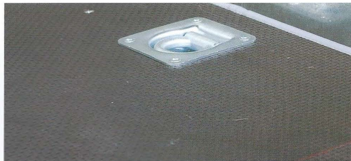
The use of a phenolic wire mesh, non-slip, overlay used for a lorry floor
